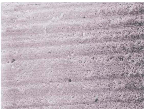
Fig. 3. Micrograph of fracture surface of Dyract specimen repaired after 10 minutes at 15 KV (500X).
