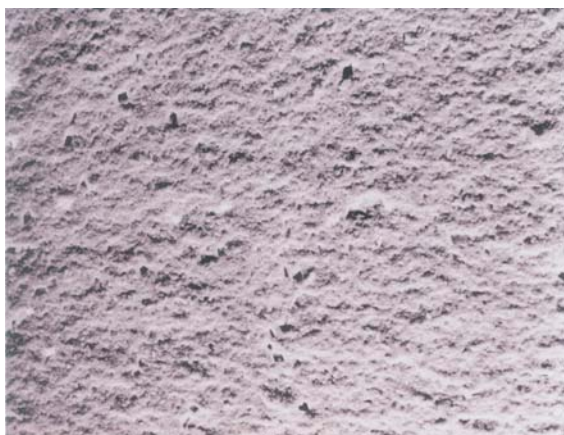
Fig. 2. Micrograph of fracture surface of Dyract control specimen at 15 KV (500X).
