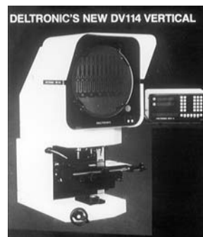
Fig. 1. The profile projector used in the study.
