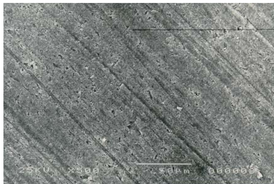
Fig. 3. Scanning electron micrograph of Dyract ® AP control, no treatment, group 2 (500x).
