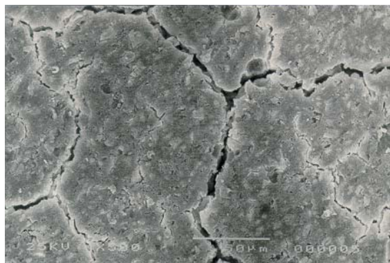
Fig. 2. Scanning electron micrograph of Ketac-Fil control, no treatment, group 1 (500x).
