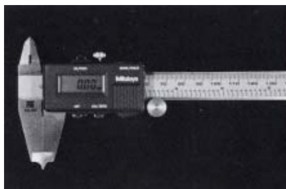
Figure 1. The electronic digital caliper with sharpened beaks to improve access interproximally.
