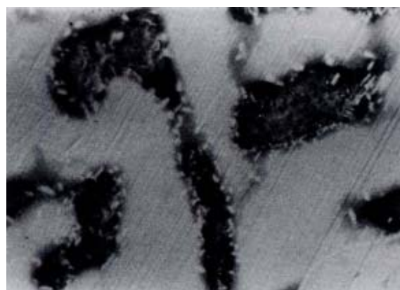
Fig. 11 Microstructure of alloy # 1 as-cast and as solution heat treated (x 1000).
