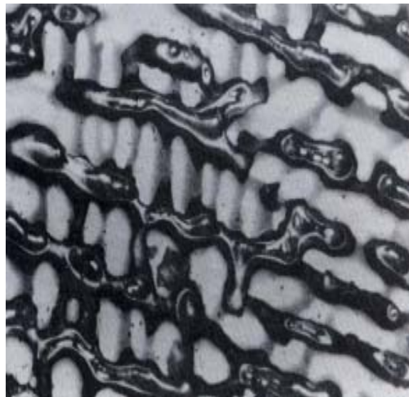
Fig. 7 Microstructure of alloy # 3 (x 400).
