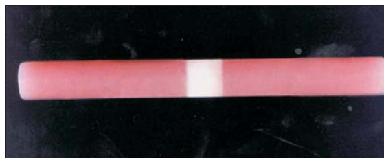
Fig. 2. A tensile test bar with a prepared tooth in its middle segment.
