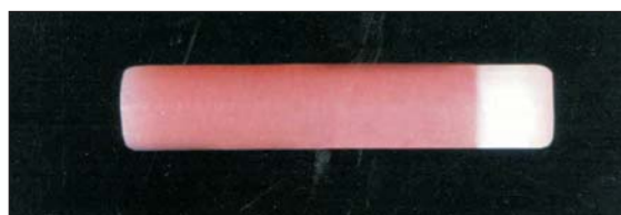
Fig. 1. Tooth ended half tensile bar prior to bonding to the second half
