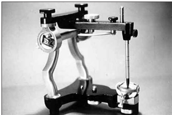
Fig. 1. Hanau H 2 158 articulator. The condylar spheres are connected by a rigid condylar shaft which can move mediolaterally within their respective condylar spheres.
