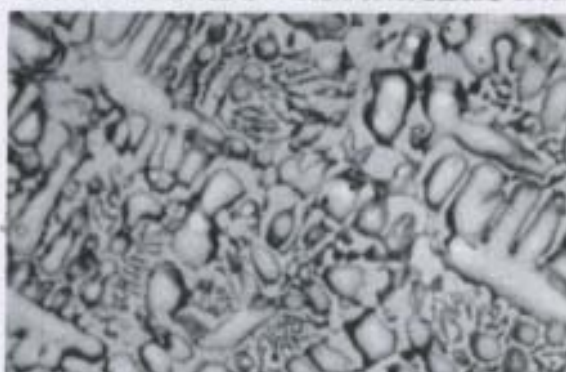
FIGURE 7. Microstructure of niobium-bearing alloys, 19.3% Nb.
